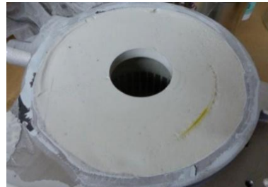
Fig.47 Final product in the case of global potting [46]
