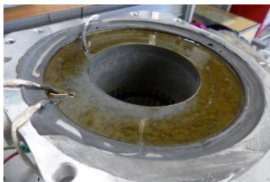
Fig.46 Final product in the case of end winding potting [46]
